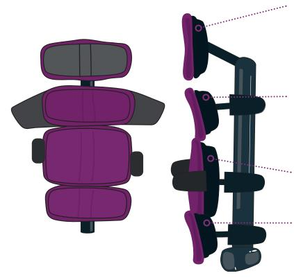
Trunk and head support: Grace requires firm trunk support to discourage kyphosis and correct scoliosis, with individualised support to improve arm function. To achieve this, a complex backrest was chosen to allow for both depth and rotational adjustment at each of its three segments.
