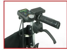
Easy-to-use controller with speed dial, battery indicator and hand controlled lever
