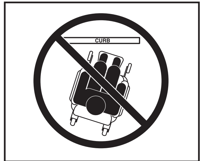
Figure 5. Incorrect Curb Approach
