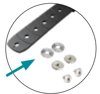
The Evoflex comes with simple, low-profile fasteners that fit into even the tightest places. New wave spring washer allows variable tension to prevent unwanted rotation and help keep belt securely attached over time.
