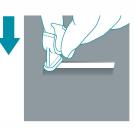
1. Locate the circular pin into the circular hole at the rear of the Caddy
