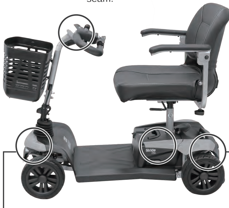
2. Use the original pry tool to open the car body along the seam.
