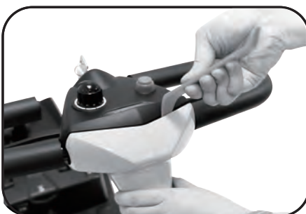
2. Use the original pry tool to open the car body along the seam.
