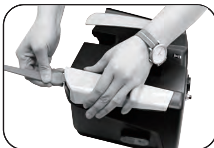
4. Remove the battery box (see 5-3 Easy Removal). Insert the pry tool into the lower seam of the trim cover and carefully remove it.
