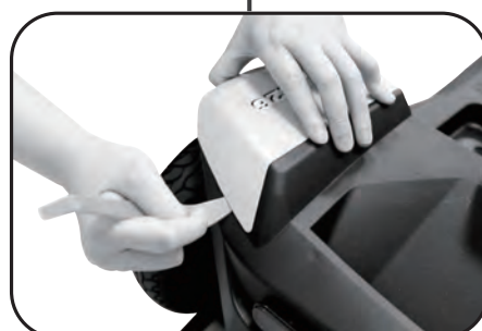
5. Insert the pry tool into the seam, pry it up, and remove it.
