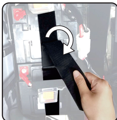
5. Loosen the Velcro to release the fixation
