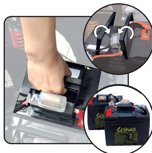
6. Remove the battery and use Just use the handle to carry it and you're done.
