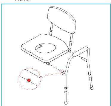
Slide the side assembly into the seat frame assembly.
