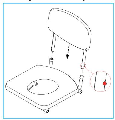
Slide the backrest assembly into the seat frame assembly.
