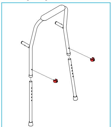
Insert the legs into the side frame and secure with 2 x E-clips.
