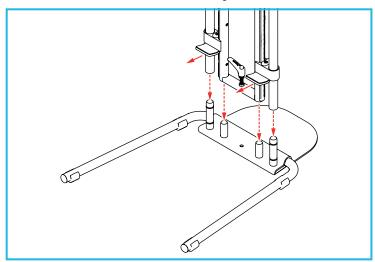
**Note:** Make sure the bed clamp plates point in the direction shown.
