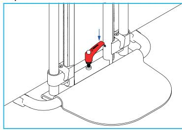
Release the tightening lever, this will re-engage the thread.
