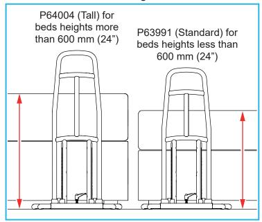
NRS recommends fitting the standard bed rail (P63991) on beds with a mattress height up to 600 mm; for higher beds, the tall bed rail (P64004) should be used.
