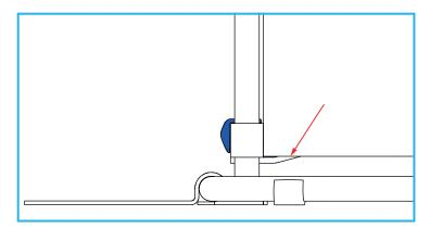
Slide the blue clamp levers outwards to unlock the ratchet clamps. While holding the clamp levers open, slide the ratchet clamps up until the clamp plates make contact with the bottom of the bed frame.
