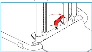
Turn the tightening lever clockwise until you start to feel slight tension. Do not over tighten as this will start to lift the handrail assembly off the base frame.
