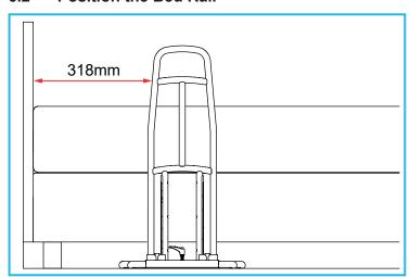
Position the bed rail so the user can reach the handrail from a laying position without having to stretch.
