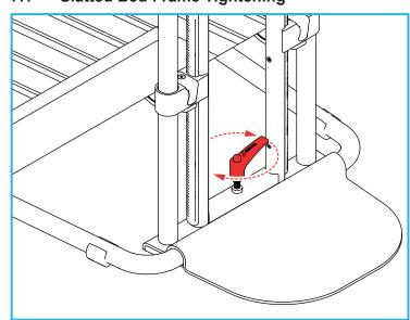
Turn the tightening lever clockwise until you start to feel tension and the bed rail feels secure.
