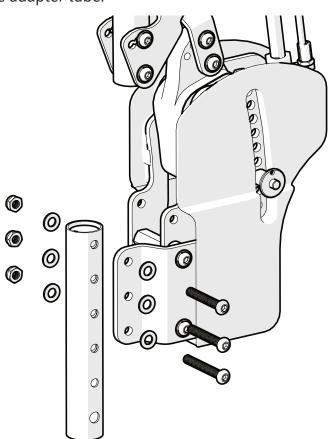
If one of the tube nuts should slide free and slip to the bottom of the adapter tube, simply release the tilt lock on that side, tilt the tube forward until the tube nut can slide back to its position. Relocate the threads with the fastener and secure the tube nut in position.
