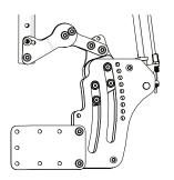
Notice in the images above, when the depth of installation is changed, the orientation of the back support canes must also be changed to retain correlation of back support to pelvic support.
