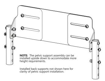
When the brackets are securely fastened to the adapter tubes, tighten the bolts securing the center plate to the torque specified.
