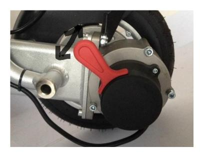
For the chair to be driven by the operator the clutch lever must be in the UP position. This engages both the electromagnetic brakes and the motors and allows the operator to drive the chair from the controller.
