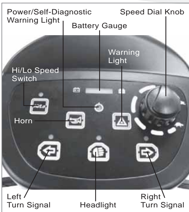
Figure 2 - HS-898 Control Panel
