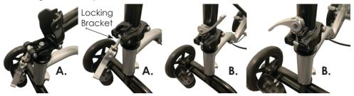
A. Push the lever to the left to disengage the pin and pull the steering column until it is in the full upright position. Now, release the handle to engage the safety pin (the steering column will stand in the upright position if the safety pin is engaged).
