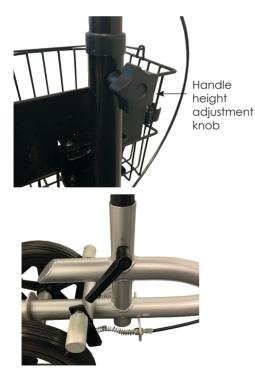
2. To adjust the handle height, loosen the handle height adjustment knob by turning it counter clockwise until it can be removed. Adjust the handle grip to the desired height and reinsert the adjustment screw into the hole, turn it clockwise until it is tightened.
