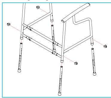
Insert the legs and set to the correct height for the toilet and user, then secure with the 4 x E-clips.
