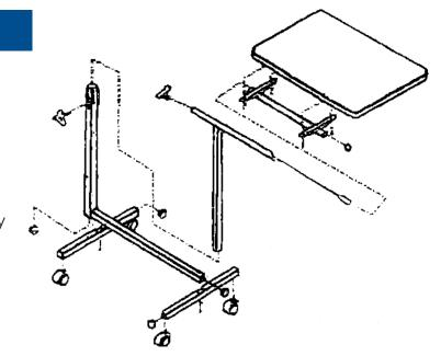
**4.** Adjust the tray to the desired inclination and tighten the tray pivot adjusting screw; set the height of the tray and tighten the main adjusting screw.
