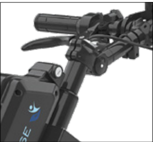
TRACK ASSISTANCE Increased driving comfort and safety The self-centring steering system straightens PAWS after release
