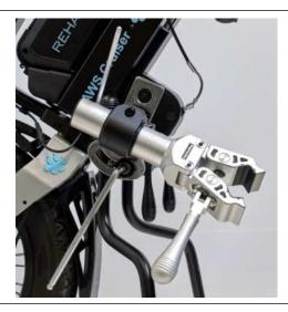
4. Loosen all three adjustment screws for height, rotation in/out and angle with a 6 mm and 8 mm Allen key so that the entire fastening part is completely loose and flexible.
