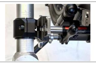
8. Adjust the width so that the clamps are the same distance from the centre of the PAWS and lock with the quick-release locks. Lock PAWS to the wheelchair, loosen the locking ring screw on each side with a 4 mm Allen key.
