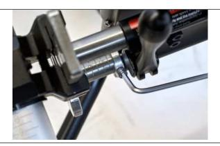
9. Insert the locking rings towards the centre of PAWS and lock them in place. This means that the entire attachment unit will be in the correct position when, for example, you have removed them carrying PAWS in the car.
