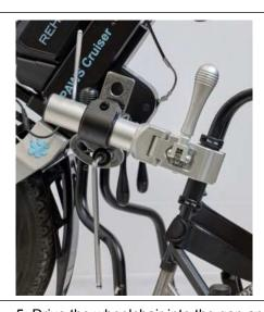
5. Drive the wheelchair into the gap and find a position to be able to lock the grip around the leg support (tube guard). When you can lock the grip, it means that all adjustment measurements are correct.
