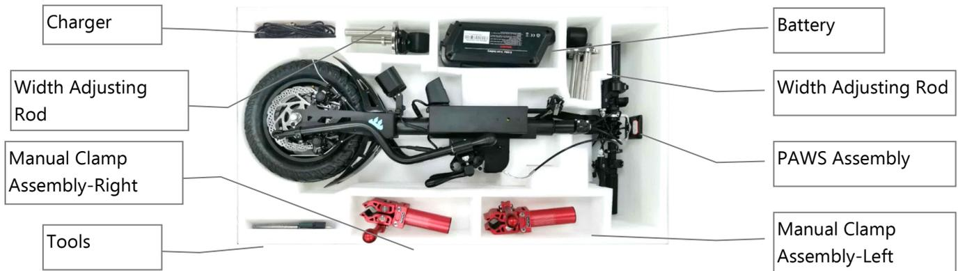
**Figure 14. Parts shown in their packing box.**
