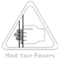
There is a risk of body part trapping during folding, unfolding, and adjusting different elements of the device. It specially concerns fingers or hands.
