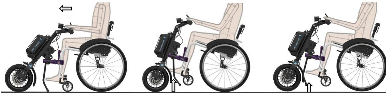
**Figure 37. Parking (1), City (3) and Touring (2) positions for Manual Clamp/Lift Devices**
