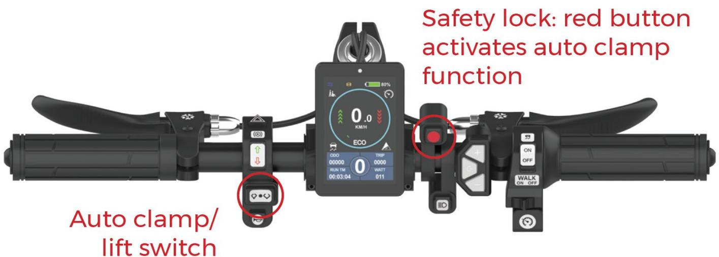
**Figure 10. Auto clamp/ lift switch**
