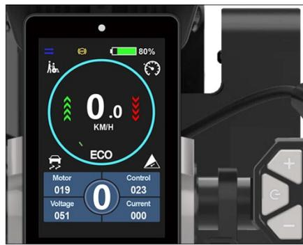
**Figure 39. Power Device and Mode Selector Buttons**
