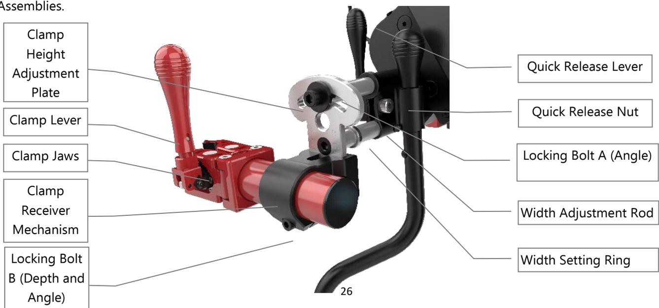
**Figure 12. Manual Clamp and Width Adjustment Assemblies**
