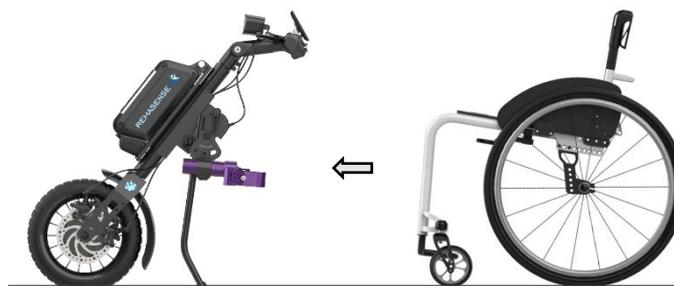
**Figure 32. Roll the Chair to the Device**
