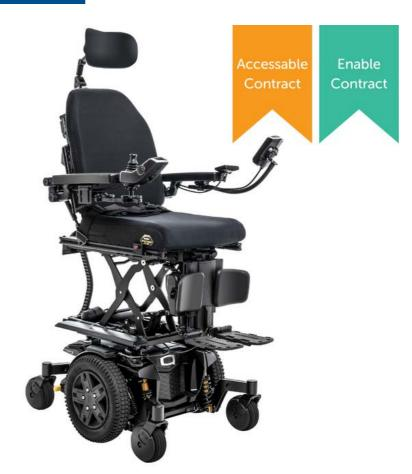
The Edge 3 combines several unique groundbreaking technologies that allow for this mid-wheel drive powerchair to perform like no other. Upgraded SRS (Smooth Ride Suspension) provides a smooth, comfortable ride and advanced stability for the user. Superior ride quality, and the ability to easily customise both the mechanical and electronic set-up, allows the user to maximise access in their home environments, and get out into the community easily.
