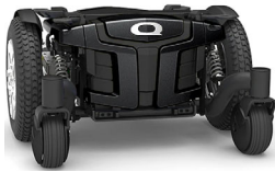
Edge HD - Mid wheel, 204kg max user weight.
