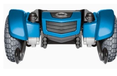
Q1450 - Front wheel, 272kg max user weight.
