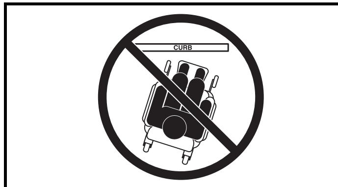
Figure 3. Incorrect Curb Approach
