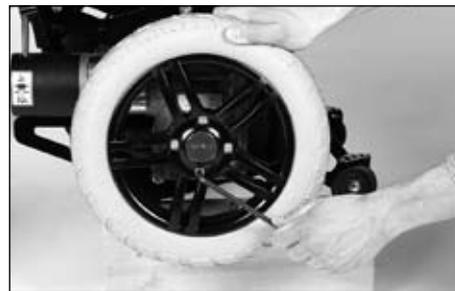
**Fig. 45** Removing the drive wheel
