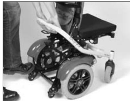
**Fig. 13** Lifting/removing the frame
