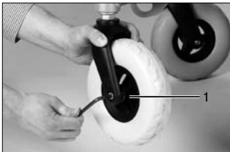
**Fig. 46** Removing the castor wheel
