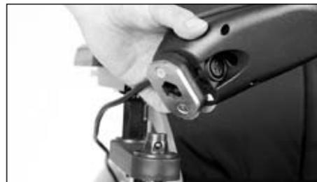
**Fig. 21** Removal for a swing-away control panel holder
