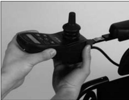
**Fig. 7** Removing the control panel
