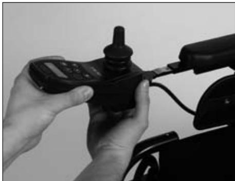
**Fig. 20** Removing the control panel
