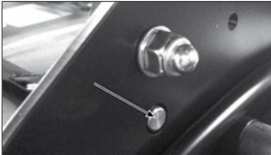
Fig. 14b Locking pin, engaged
