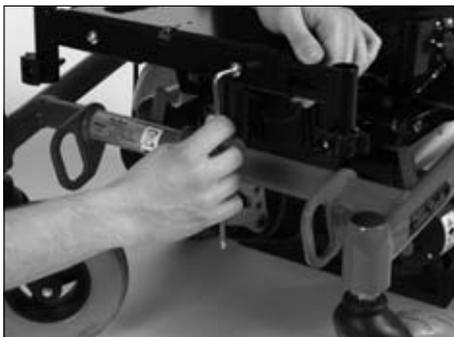
Fig. 26 Footrest holder: Adjusting the lateral position
