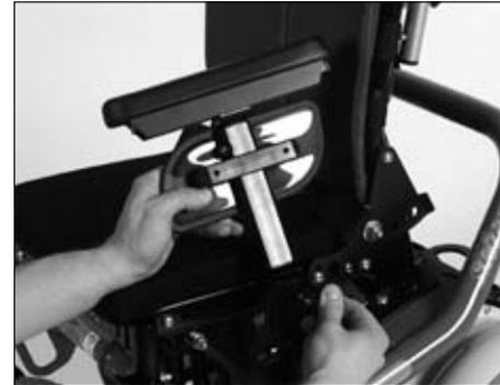
**Fig. 17** Removing the side panel
