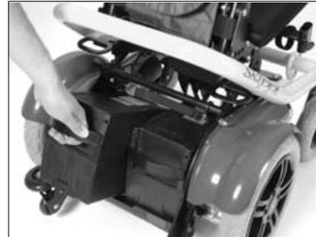
**Fig. 11** Removing the battery packs
