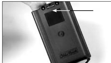
Fig. 44 Battery pack with fuse
