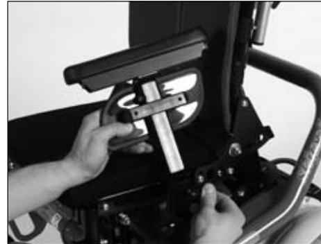
**Fig. 8** Removing the side panels
