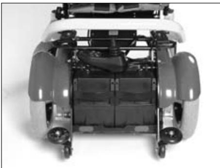
**Fig. 12** Push the step points (frame protection rollers) down
