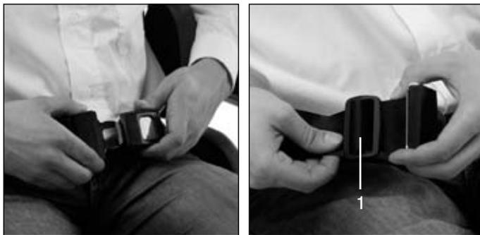
**Fig. 43** Applying the lap belt
