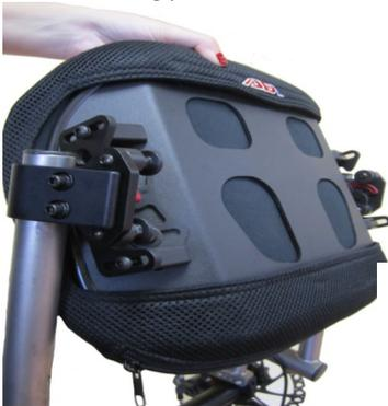
2. After bottom hooks are in position, tilt back support rearward until top hooks are fully engaged onto top receiving posts.
