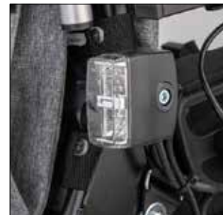
ES 06 Four way lighting, at the back
